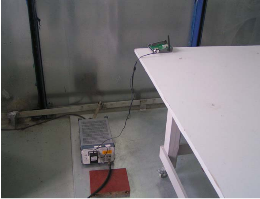
Conducted Emission Test Set-up View
