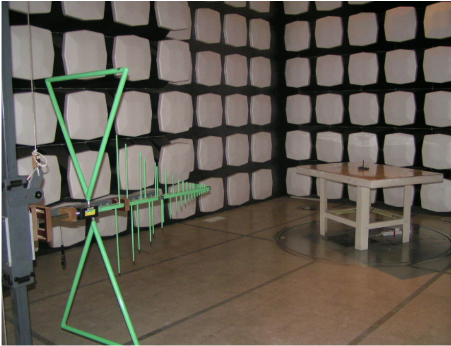
Fundamental & Harmonics Strength Test Set-up View - Low Frequency
