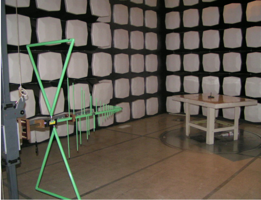
Radiated Emission Strength Test Set-up View - Low Frequency
