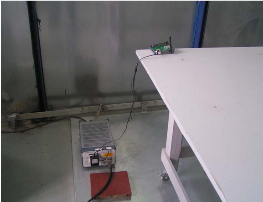
Conducted Emission Test Set-up View
