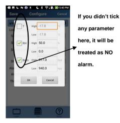
For example: Temp. is marked, High is 8  $^\circ\!C$  and Low is 2  $^\circ\!C$ , it means that an alarm condition will occur below 2  $^\circ\!C$ , or above 8  $^\circ\!C$ . The programmable alarm limit of each parameter is
