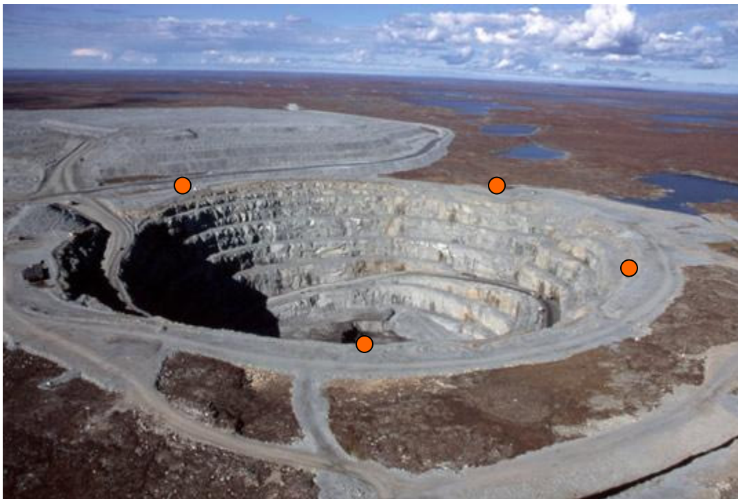
Figure 1: An open pit mine with a typical deployment (orange dots) of the TX100 transmitters. The above is a scenario only illustrating transmitter positioning. Double-benching is being used, making each “step” a 100 feet tall.
