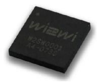
The device integrates all the circuitry necessary for wireless in a single package with the exception of an external antenna. The W2SW0001C-T is a complete system-in-package which includes the Marvell 88W8686 802.11b/g chip set, crystal, power amplifier and filter components. The internal crystal oscillator operates at 26 MHz frequency (frequency stability +/- 20 ppm) and requires no external clock source. A pin provides the antenna interface with 50 Ohm impedance.
