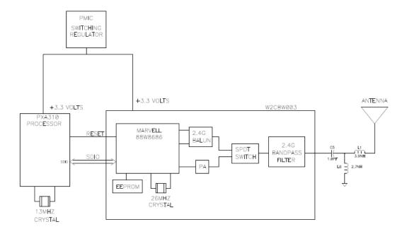
The transceiver uses Orthogonal Frequency Division Multiplexing (OFDM) and Complementary Code Keying (CCK) modulation for the 802.11b/g. The antenna is a surface mount chip antenna manufactured by Fractus, part number FR05-S1-N-0-00.1. The Fractus antenna has a gain of approximately 2.0 dBi.
