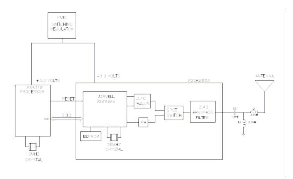
The transceiver uses Orthogonal Frequency Division Multiplexing (OFDM) and Complementary Code Keying (CCK) modulation for the 802.11b/g. The antenna is a surface mount chip antenna manufactured by Johanson Technologies, part number 2450AT18A100E.
