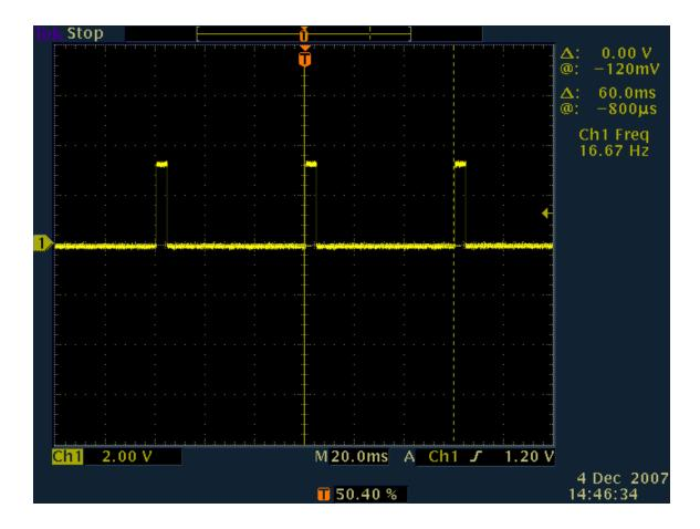
The following screen shot shows the duration the transmitter is active. This time is approximately 4.3 milliseconds. After the master device transmits a message, it waits for a response from a slave device. Each message contains an address to identify which slave device should respond. Each message also contains a 16-bit CRC to ensure corrupt data will not cause more than one slave to reply.
