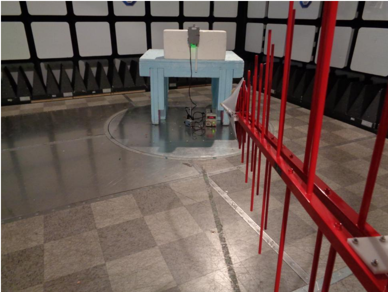
Photo 3: – Test Setup – 30MHz to 1GHz – Vertical Polarization
