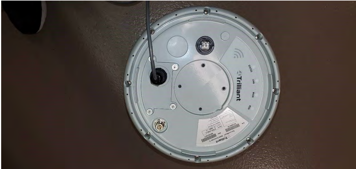
Figure 31: Bottom of unit showing DC connector and 3-pin connector on the surge suppressor door.
