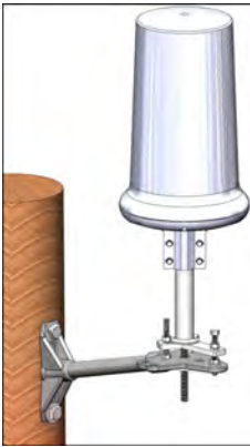
Figure 37: Typical installation: XBRG-2040-x/GWBR-2040-x mounted on pole
