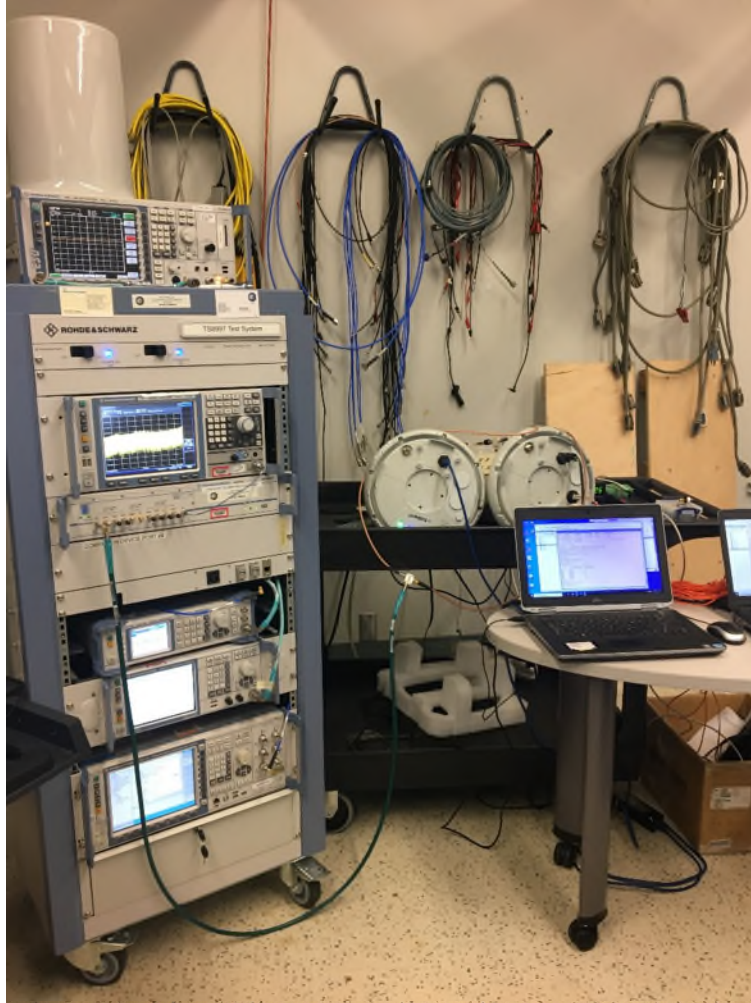
Figure 3 – Antenna port conducted emissions
