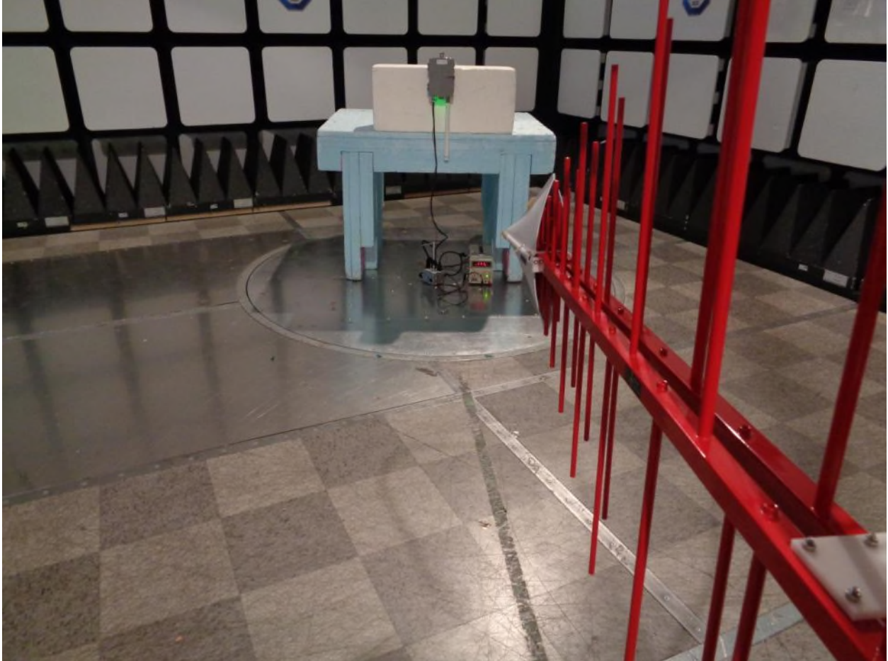
Figure 2 – Radiated Emissions Setup – 30 MHz to 1 GHz
