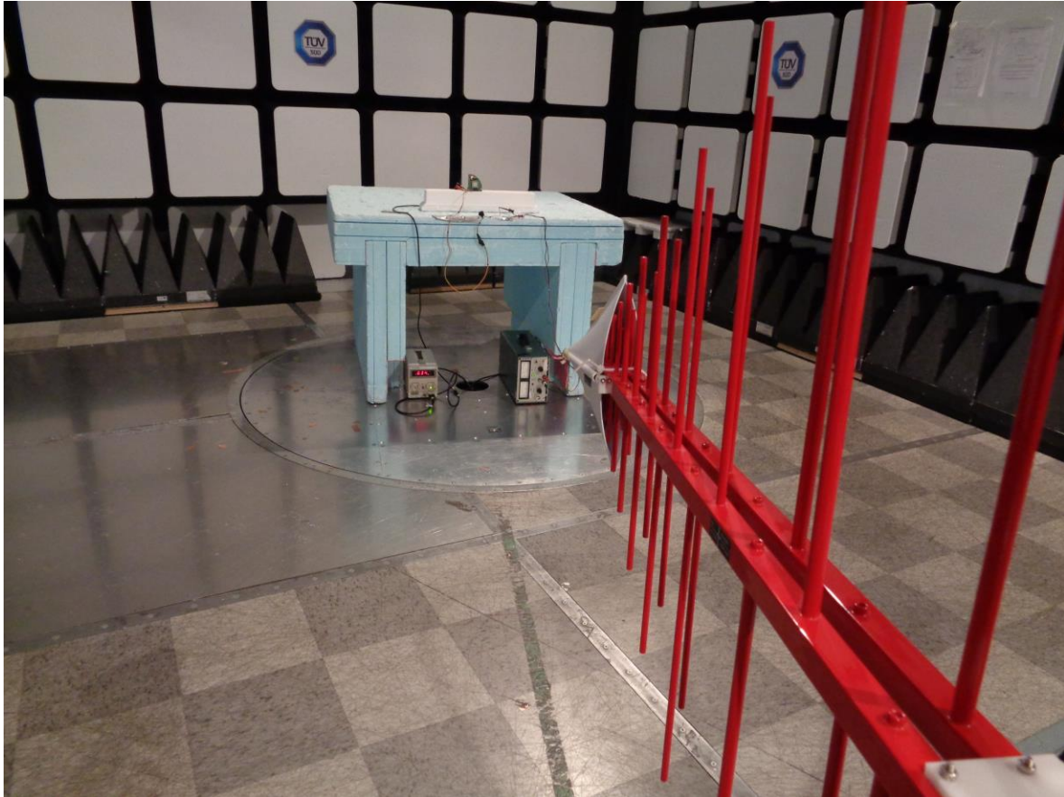
Figure 4 – Radiated Emissions Setup – - 30 MHz to 1 GHz
