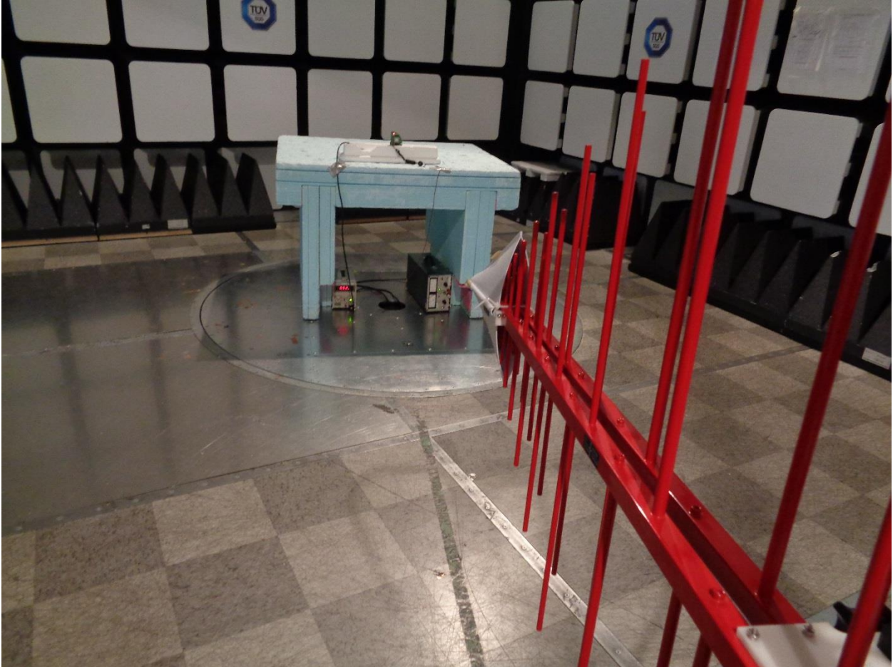
Figure 2 – Radiated Emissions Setup – 30 MHz to 1 GHz
