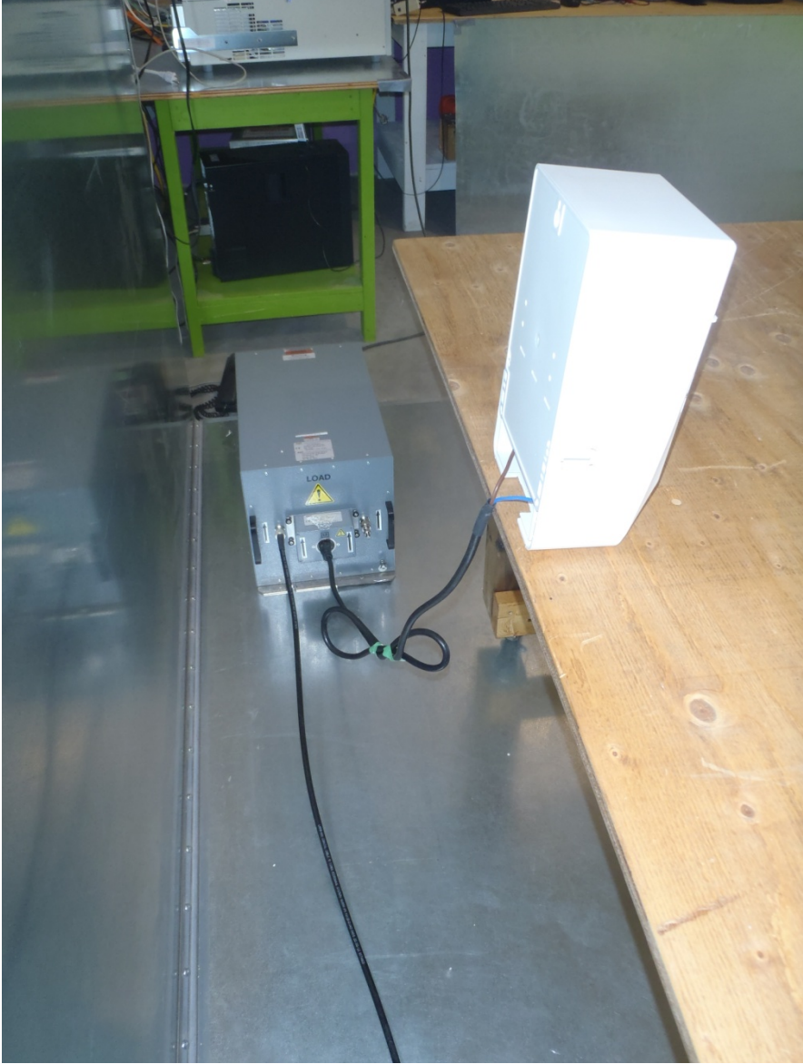
Power Line Conducted Emissions #2(in typical host SGM-3033 meter)
