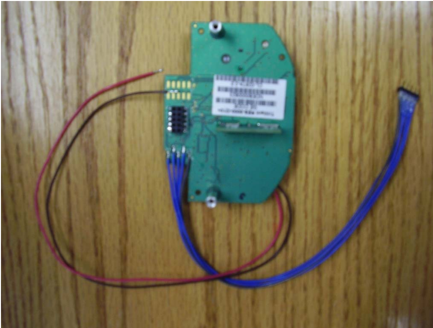
Opposite side of the radio board, showing power wires and a 5-pin connector. The antenna is nearly centered and the perpendicular PCB (near the model number and serial number label).
