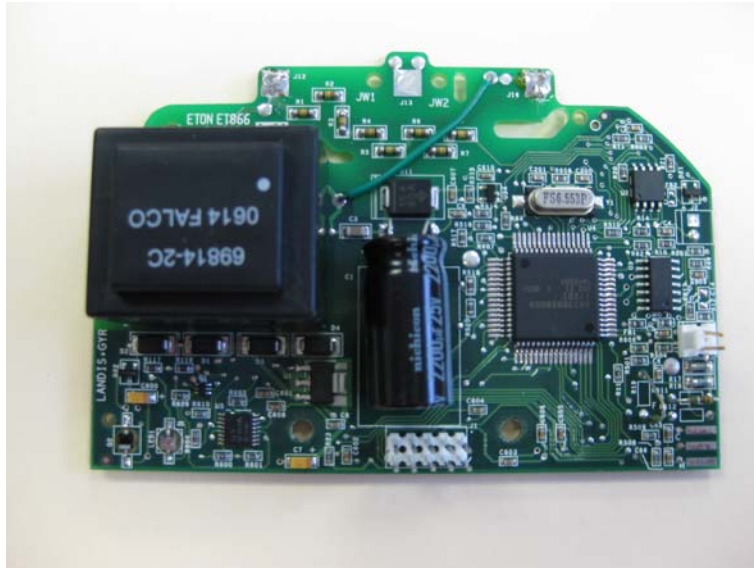
Front Side Non-RF Board for RES-3000-FOCUS
