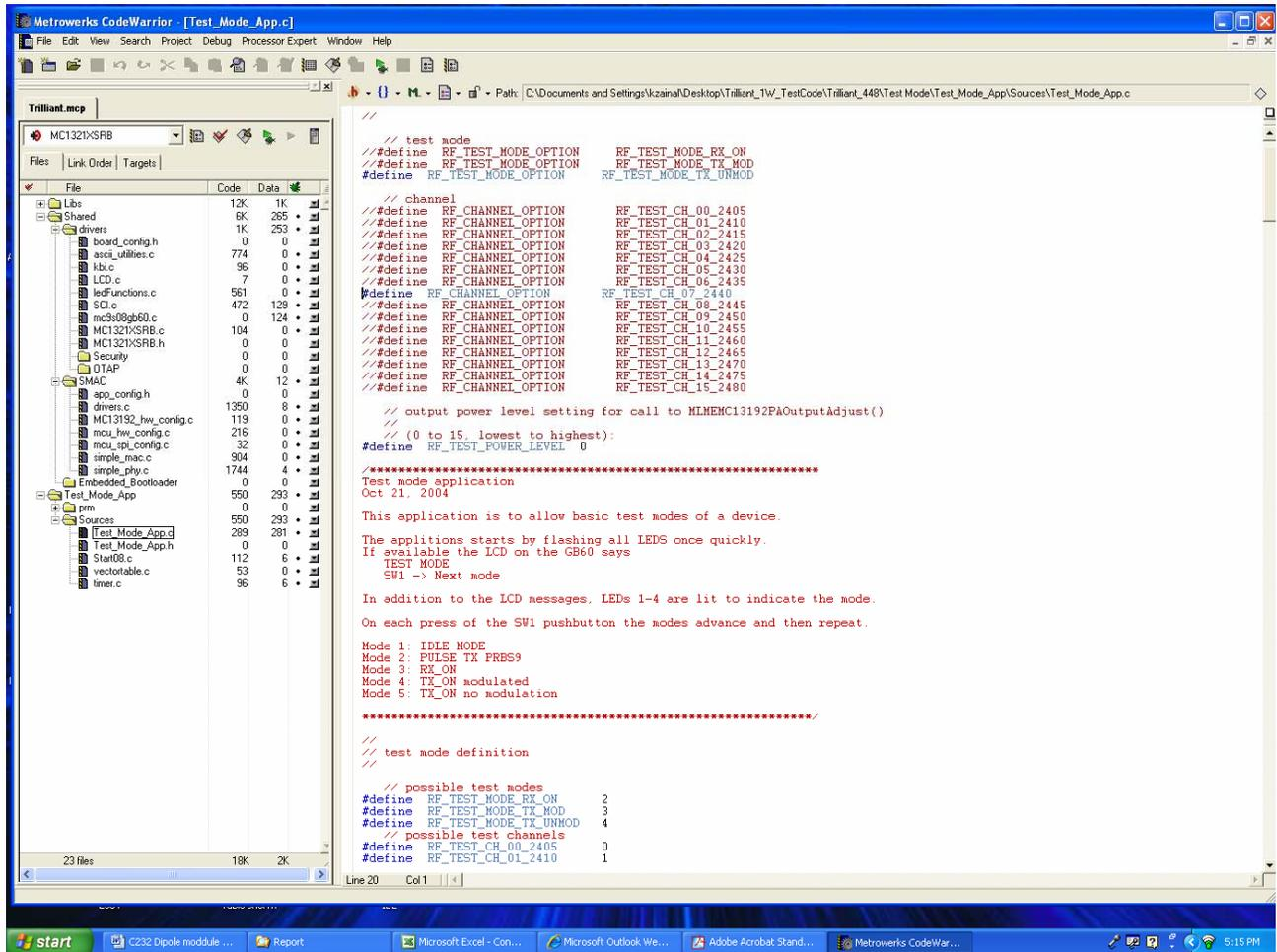
To set channels and power profile, the tester will need to activate the appropriate C commands and recompiling the C code.
