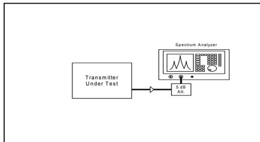
**Measured RF Power Output (in Watts): 0.977 watts**
