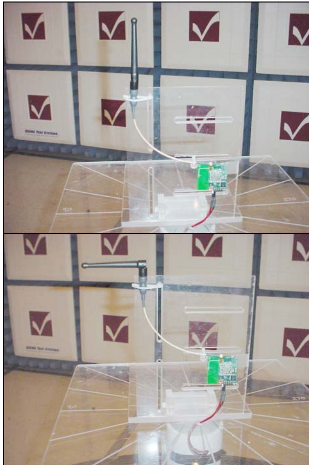
View of the EUT setup, with the Whip antenna, with EUT in vertical orientation.
