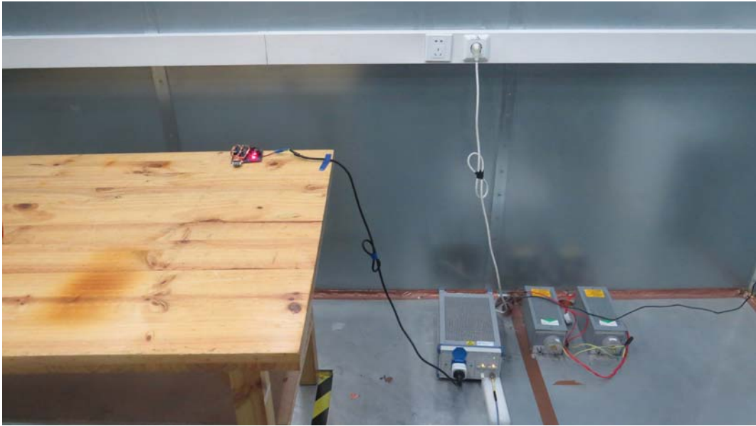
Picture 3 Conducted Emission Test Setup
