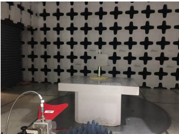
Radiated Emissions Above 1GHz - Front View
