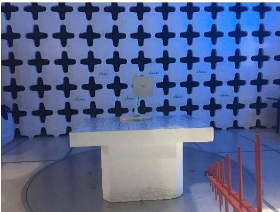
Radiated Emissions 30-1000MHz - Front View
