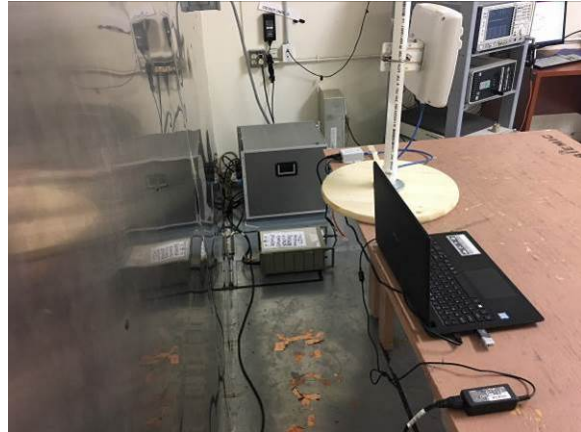
Conducted Emission - Rear View
