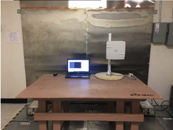
Conducted Emission - Front View
