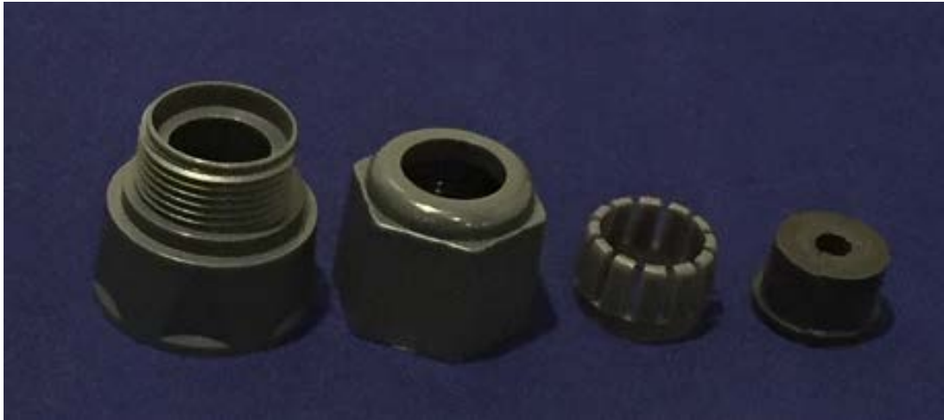
Figure 4: Dismantled Ethernet Cable Gland
