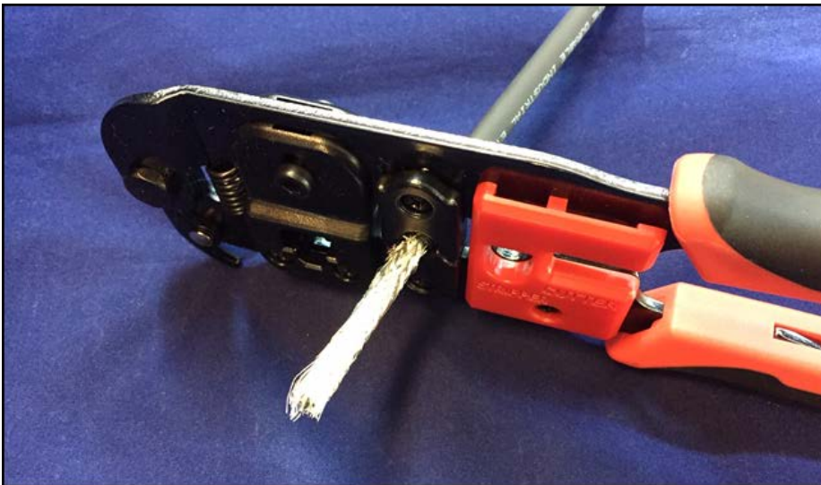
Figure 22: Crimping the Cable Strain
