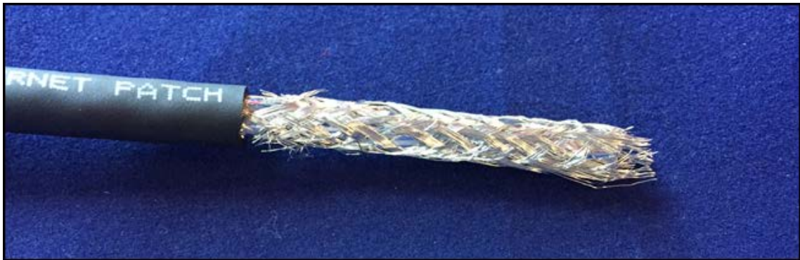
Figure 18: The Stripped Outer Jacket
