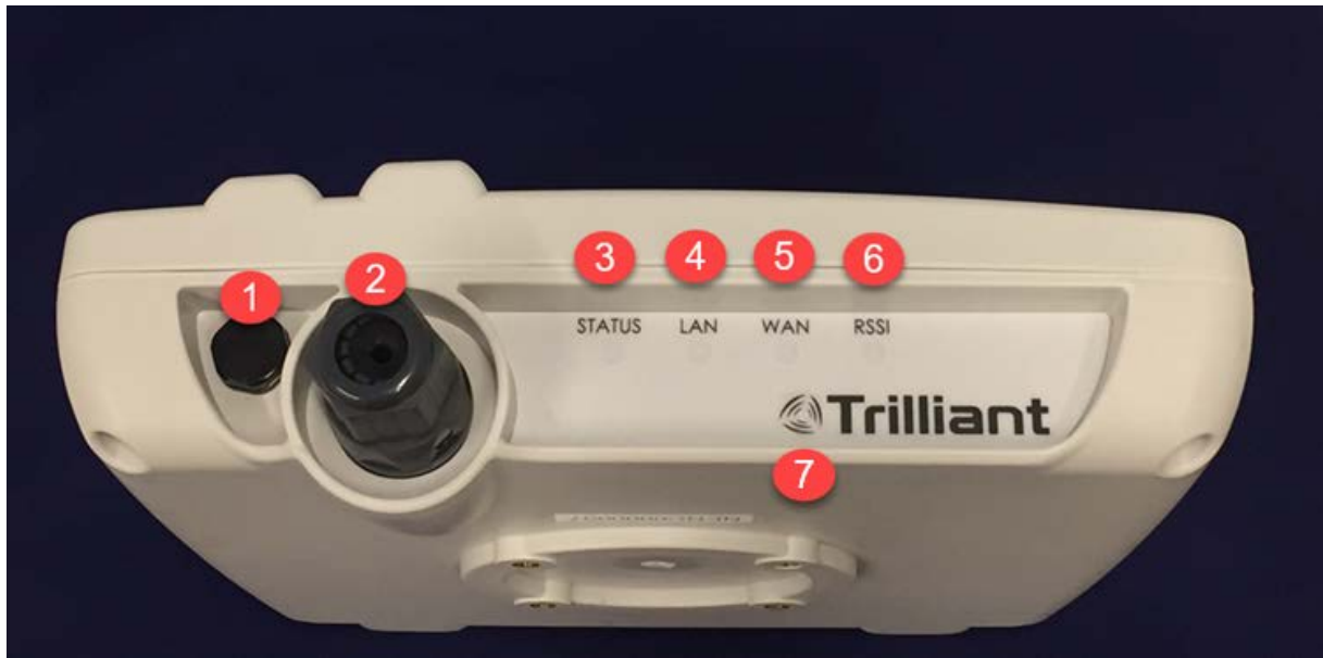
Figure 15: The CONN-2000 with the Attached Ethernet Cable Gland
