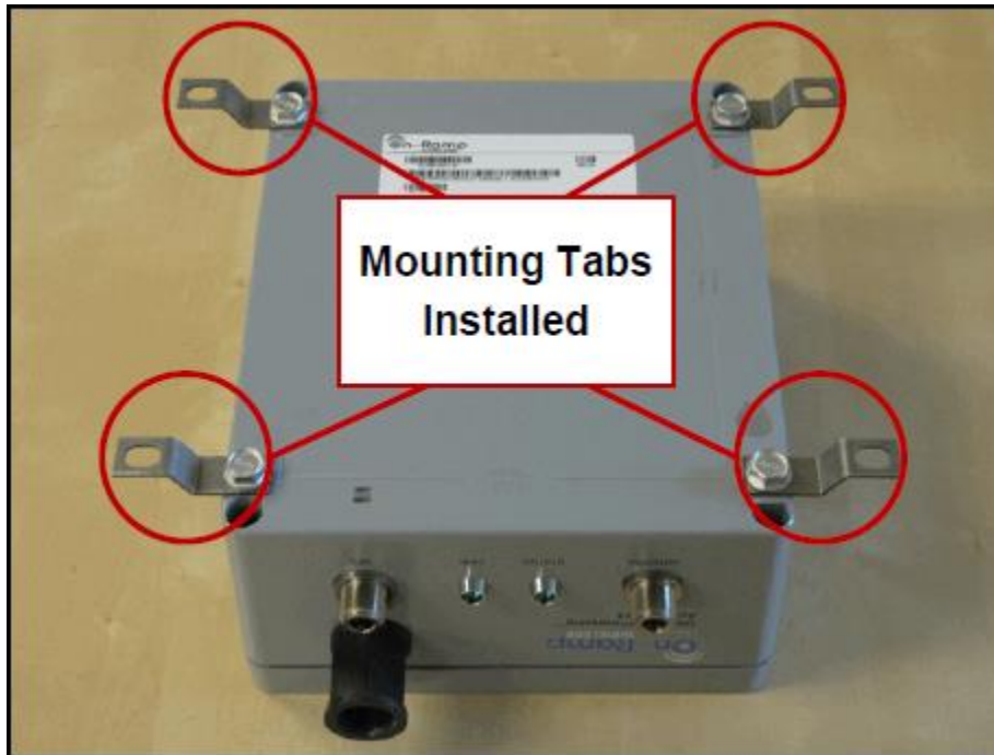
Figure 10. AP with Mounting Tabs Installed
