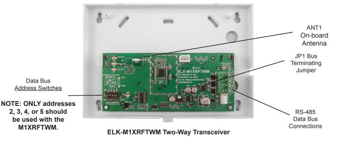
NOTE: Jumper JP1makes it convenient to terminate the RS-485 Data Bus if this is the last installed device.
