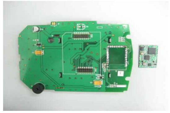
Internal View of EUT – 4(RF Module)
