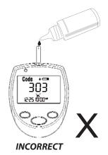
CAUTION! To avoid contaminating the control solution with the content of the test strip, you have to place a drop of control solution on a clean surface or on your finger tip first. Do not directly apply control solution into a strip.
