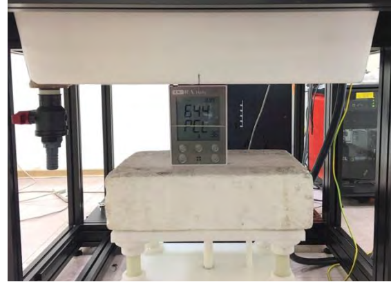
Fig.6 EUT Top-2 side to flat phantom
