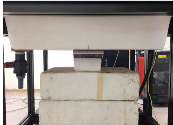
Fig.3 EUT Back side to flat phantom
