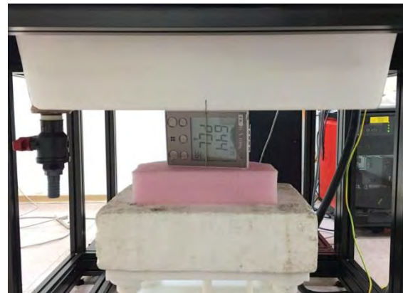
Fig.8 EUT Left side to flat phantom
