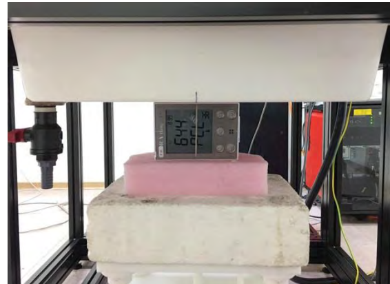
Fig.7 EUT Right side to flat phantom
