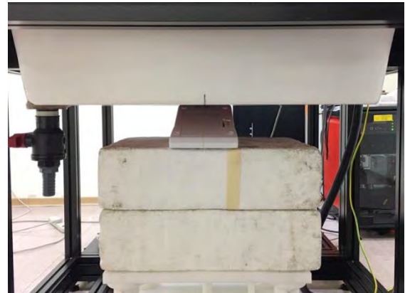
Fig.4 EUT Back-1 side to flat phantom
