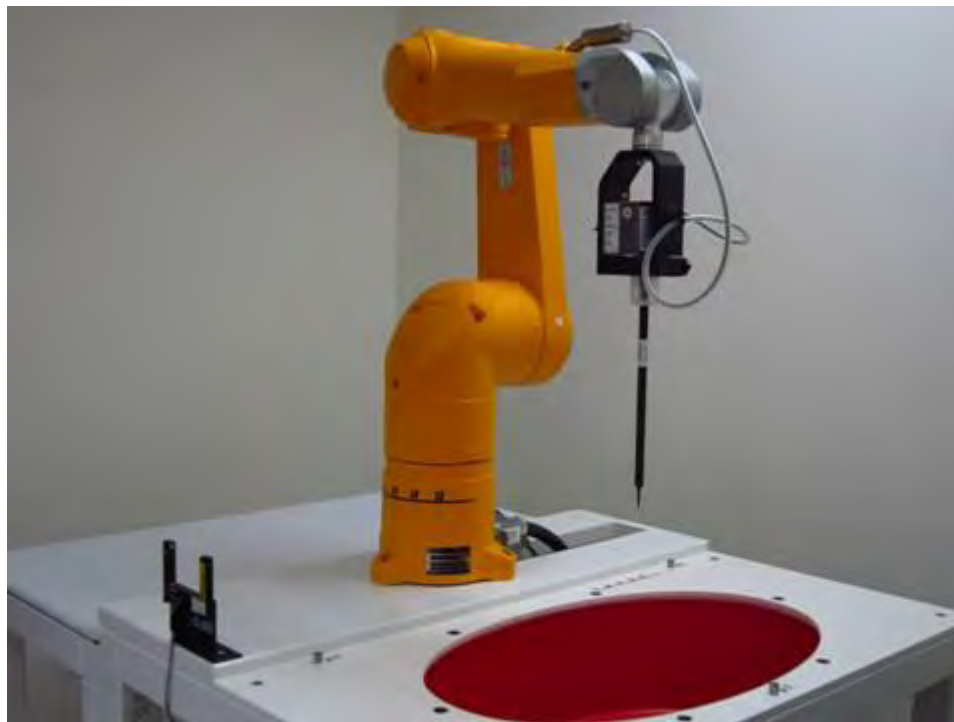
Fig.1 Photograph of the SAR measurement system
