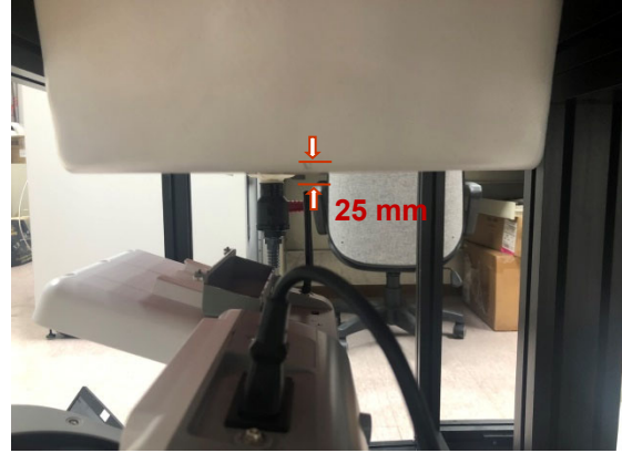
Photograph 2. Body, Top Edge of Antenna, 25mm
