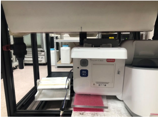
Photograph 7. Body, Back Edge of Antenna, 25mm
