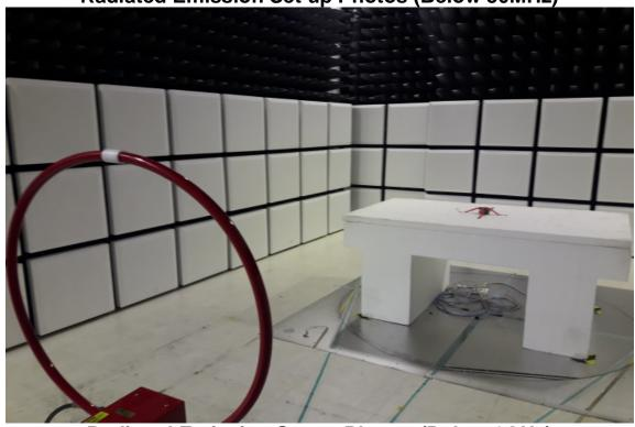
Radiated Emission Set up Photos (Below 1GHz)
