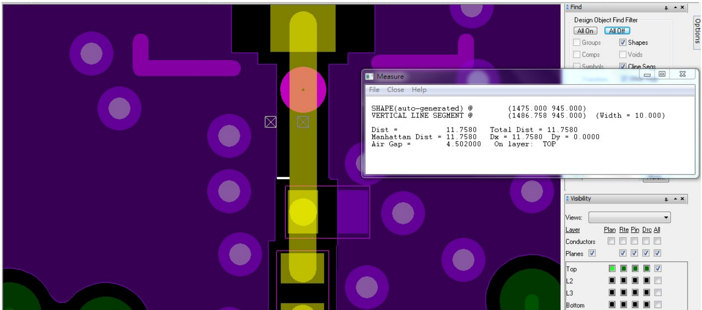
c. Air gap between RF trace and ground about 4.5 mil
