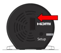
AW-WH036T's HDMI connector to media source and AW-WH036R's HDMI connector to flat panel display by HDMI cables
