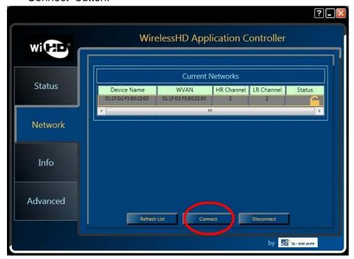
6. WirelessHD network will be linked and display the indicator of connection. The video on local notebook will be displayed on the TV or HDMI monitor connected with WiHD receiver.
