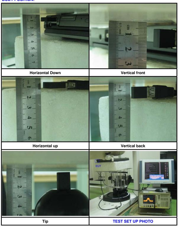
**NOTE:** The EUT face to the phantom with 5mm-separation distance.
