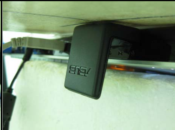
B: The bottom of the EUT faces to the phantom with 0mm-separation distance.
