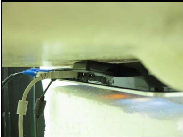
E: The bottom of the EUT faces to the phantom with 0mm-separation distance.
