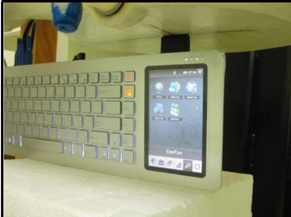
C: The edge of the EUT faces to the phantom with 0mm-separation distance.
