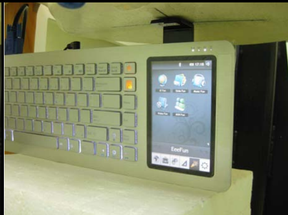
D: The edge of the EUT faces to the phantom with 0mm-separation distance.
