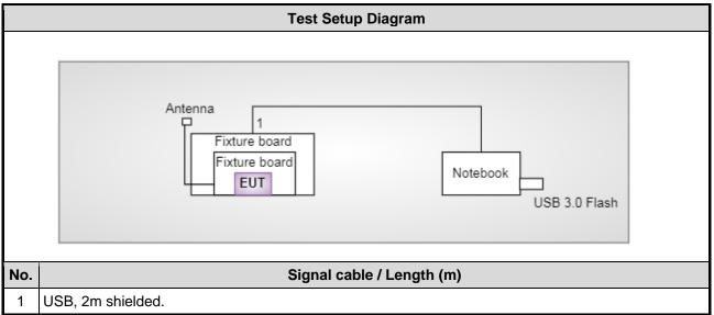
Note: The SDIO fixture is disconnected from EUT and removed from test table when EUT is set to transmit continuously
