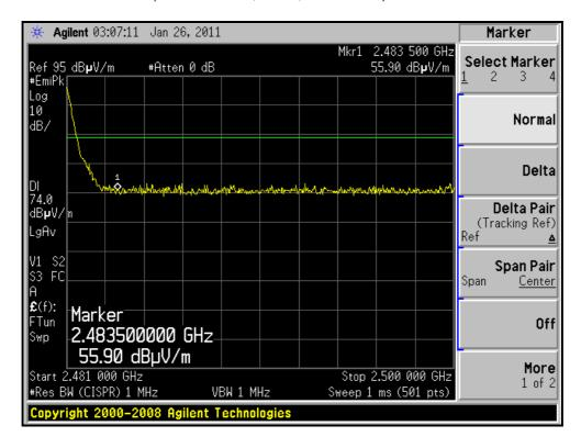
\* The average value of fundamental frequency is: Average value = peak reading + 20log(duty cycle).
