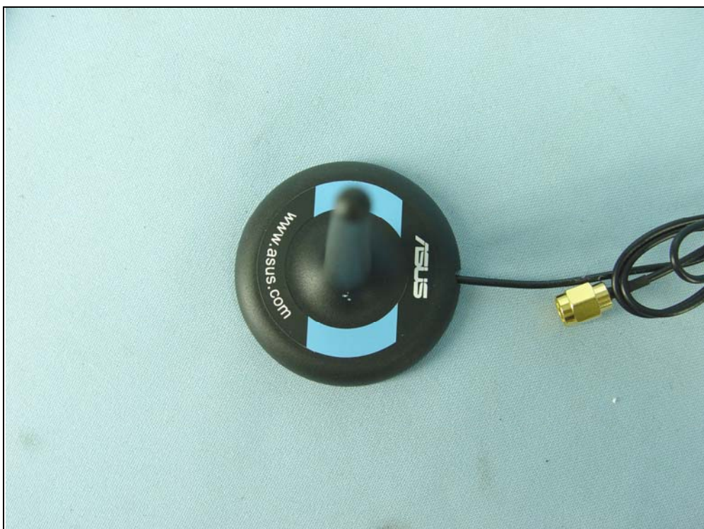
Antenna 2 (Model no.: AB006AQ-0175R)
