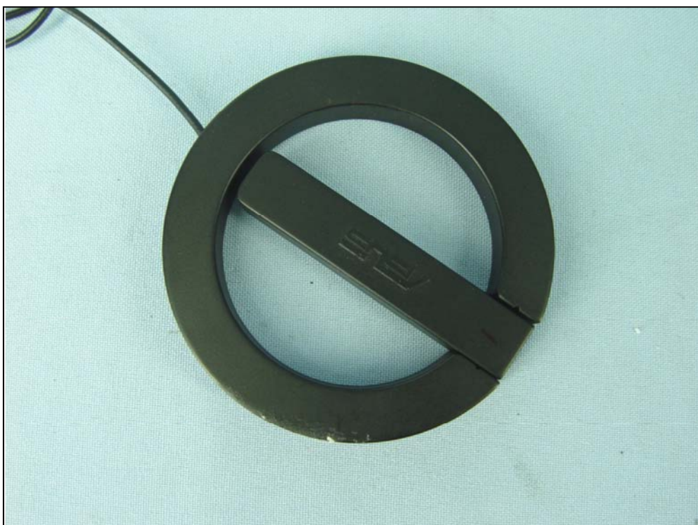
Antenna 1 (Model no.: AB006AQ-179R)
