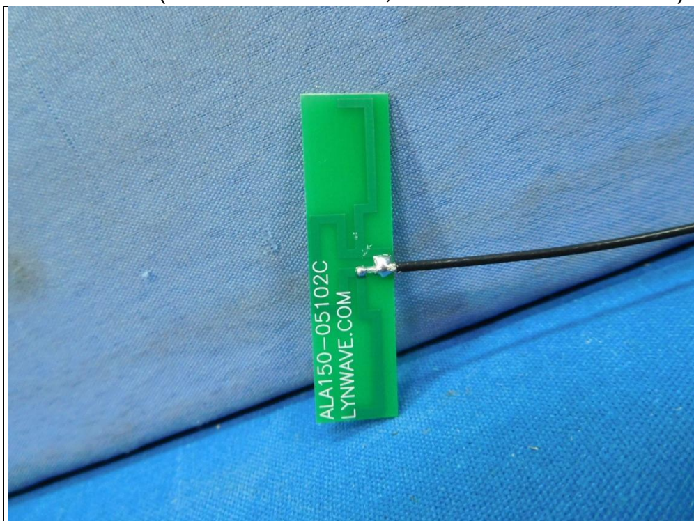
Antenna 31 (Brand: LYNWAVE ; Model: ALA150-05102C)
