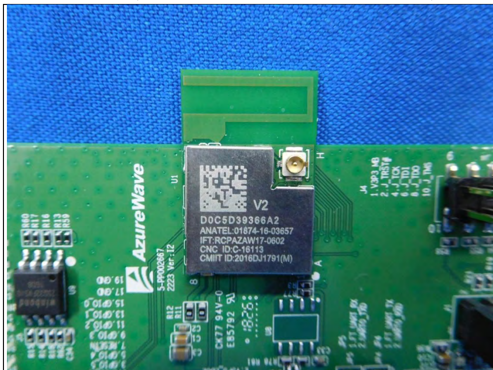
Antenna 1 (Brand: AzureWave ; Model: AW-CU300 ANT)
