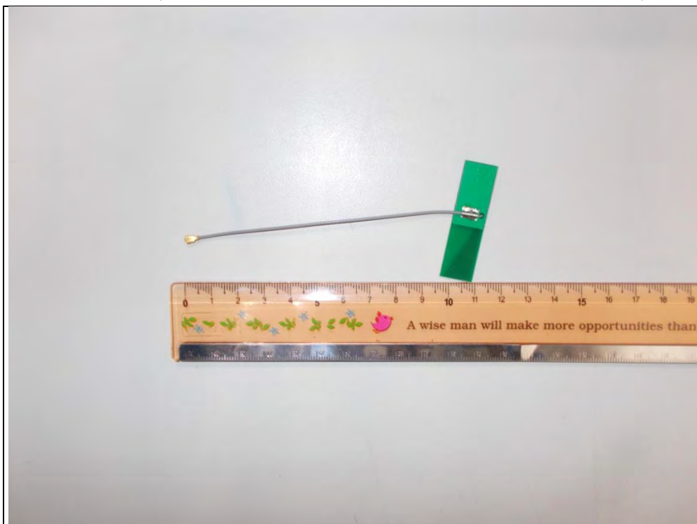
Antenna 7 (Brand: LAIRD ; Model: NanoBlue-IP04_MAF94045)
