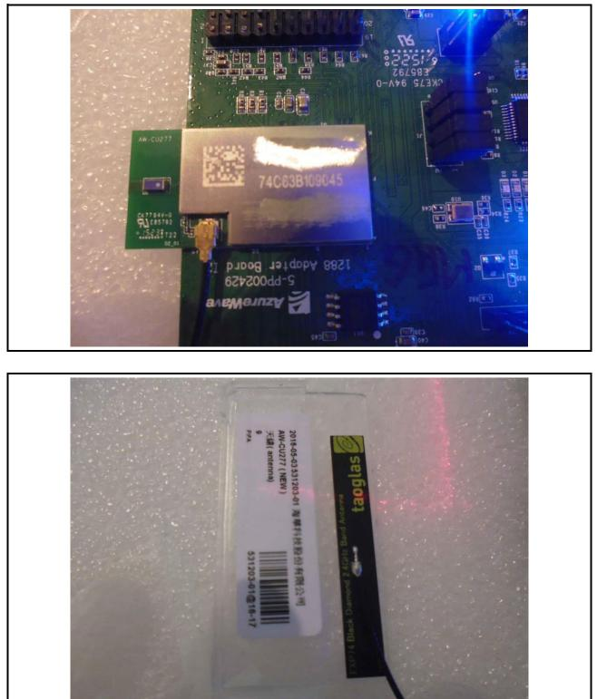
Radiated Emission Below 1GHz Test (PIFA Antenna)
