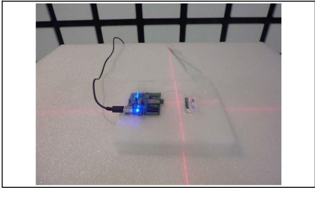
Radiated Emission Above 1GHz Test (Monopole Antenna)
