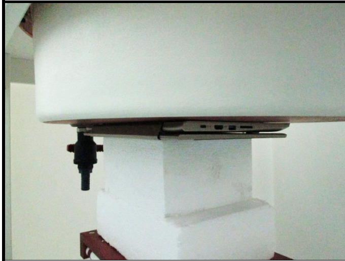
Rear Face of EUT with 0 cm Gap
