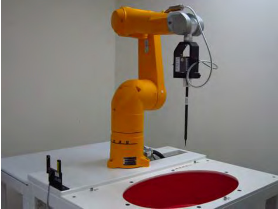
Fig.1 Photograph of the SAR measurement system
