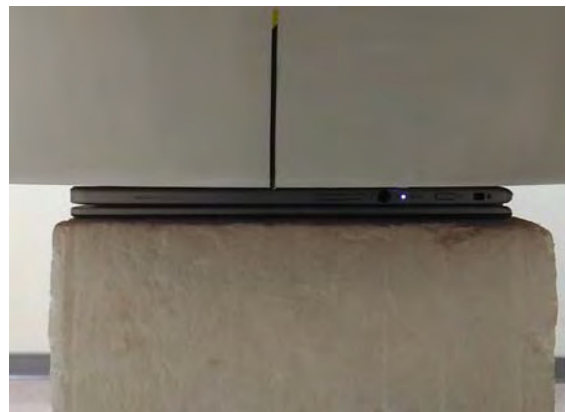
Fig.4 EUT Back side to flat phantom (tablet mode)
