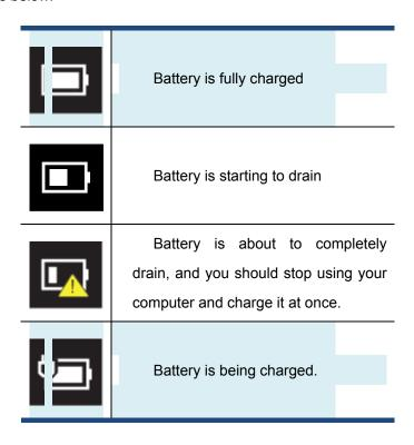
A battery is an expendable supply, so when using it over a long time, the capacity/battery life is shortened. If the battery life is reduced to under half of its initial time, we recommend purchasing a new battery.
