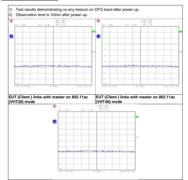
EUT (Client ) links with master on 802.11ac (VHT80) mode
