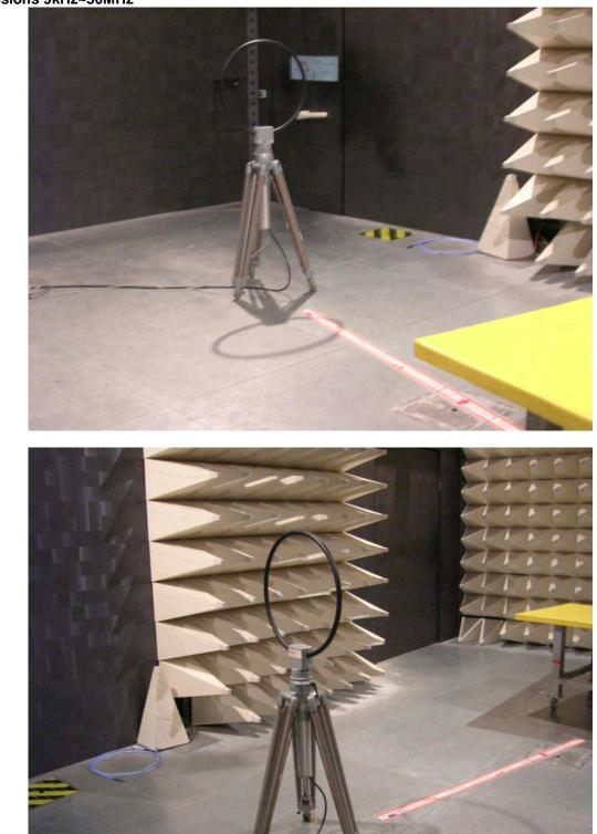
2 Photographs of Radiated Emissions Test Configuration For radiated emissions 9kHz~30MHz
