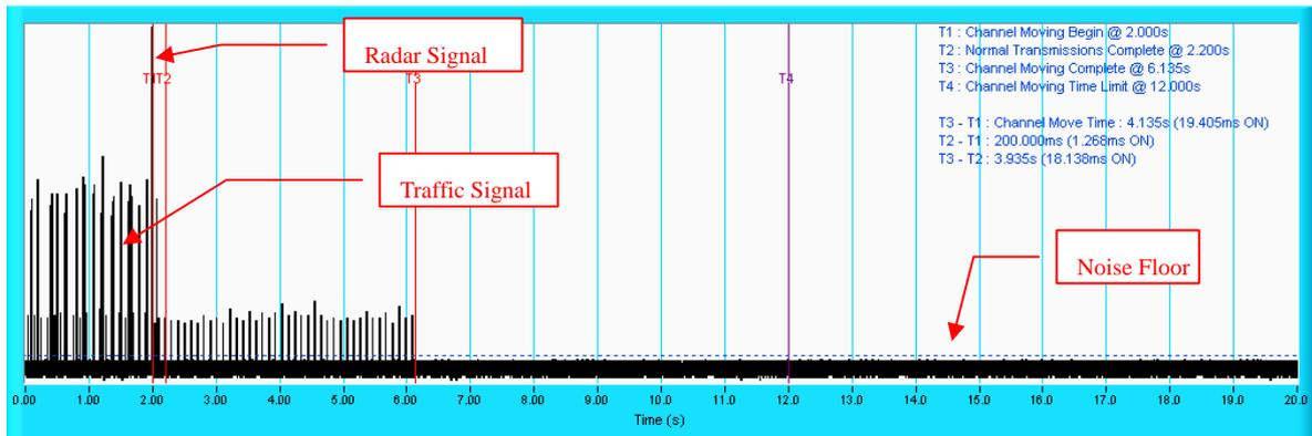
**NOTE:** T1 denotes the start of Channel Move Time upon the end of the last Radar burst. T2 denotes the data transmission time of 200ms from T1. T3 denotes the end of Channel Move Time. T4 denotes the 10 second from T1 to observe the aggregate duration of transmissions.
