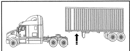
1. Raise the container with its support through radio control.
