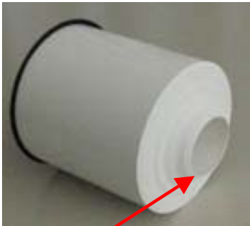
Check for uneven ends
