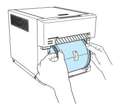
9 Remove the seal, place a hand on the paper, and rotate the paper holder in the direction of the arrow to insert the paper leading edge until the buzzer beeps.
