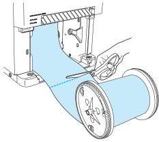
2 Remove the ribbon, insert a hand, and then grip the leading edge of the paper and pull it out toward you (direction of the arrow in the figure on the right).
