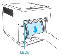
10 Attach the printer unit's trash box.
