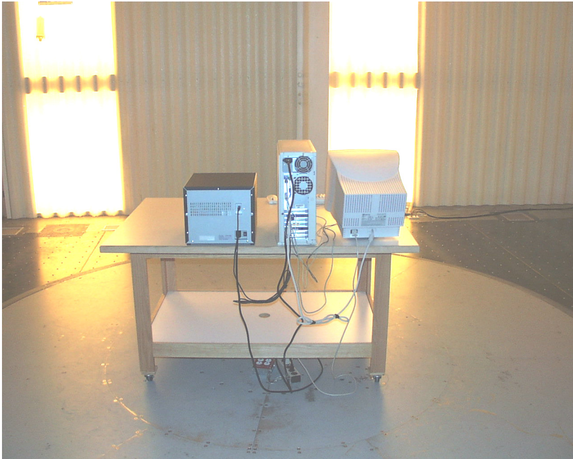
Photograph 2 - Back View of the Radiated Emissions Testing Setup
