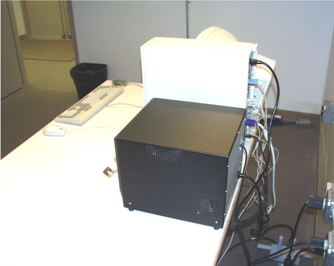
Photograph 4 - Back/Side View of the Conducted Emissions Testing Setup
