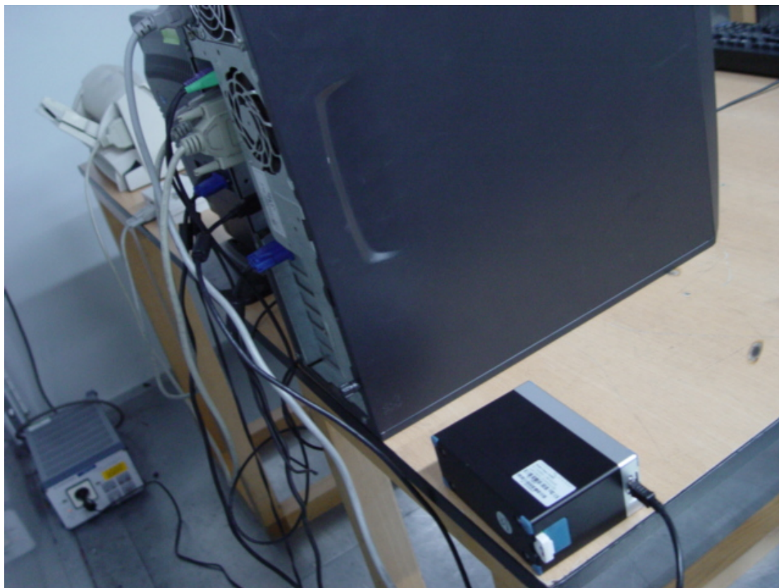
Photo 2 Conducted Emission test
